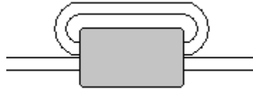
140 Ohm @ 100MHz ferrite
